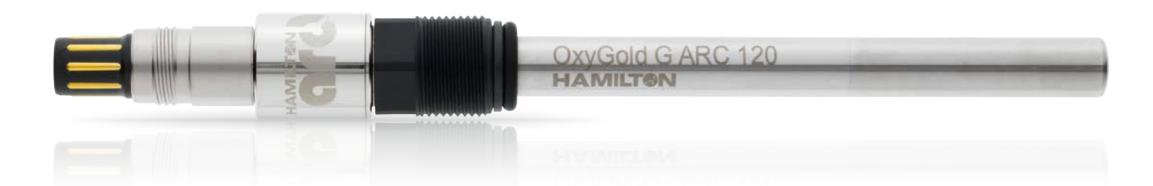
**Specifications** Measuring range 1 ppb to 40 ppm (DO) Response time t98% < 60 s at 25 °C, from air to nitrogen 0 to 130 °C (Arc: analog 0 to 110 °C, Process temperature digital 0 to 130 °C) Pressure range 0 to 12 bar (relative to ambient) Autoclavable, CIP, SIP Hygienic aspects Electrolyte Oxylyte G Surface Quality  $R_a < 0.4 \mu m (N5)$ Current in air at 25°C 180 to 500 nA Material Stainless steel 1.4435 -670 mV Polarization voltage O-ring **EPDM**
