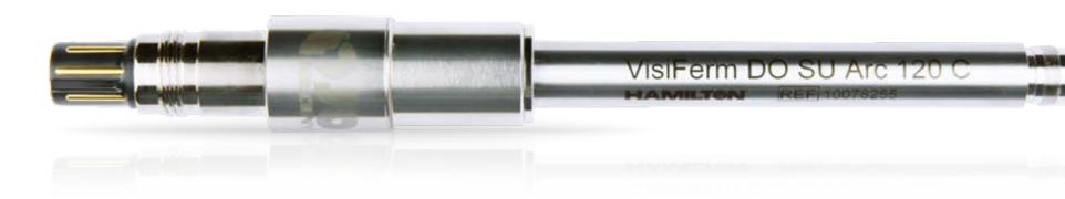
**Specifications** Measuring range 4 ppb to 25 ppm (DO) Measurement Principle Oxygen dependent luminescence quenching Response time t98% < 30 s at 25 °C, from air to nitrogen Process temperature 4 to 50 °C Operating voltage 7 to 30 VDC max. 1 W Hygienic aspects Gamma irradiation up to 50 kGy (for the disposables) O-ring **EPDM**
