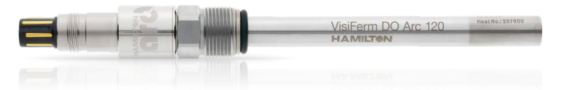
Measurement Principle Oxygen dependent luminescence quenching < 30 s at 25 °C, from air to nitrogen Response time t98% Process temperature -10 to 140 °C, the sensor provides no DO reading above 85 °C Operating voltage 7 to 30 VDC max. 1 W Pressure range -1 to 12 bar (relative to ambient) Hygienic aspects Autoclavable, CIP, SIP Surface Quality  $R_a < 0.4 \mu m (N5)$ Material Stainless steel 1.4435 O-ring **EPDM**
