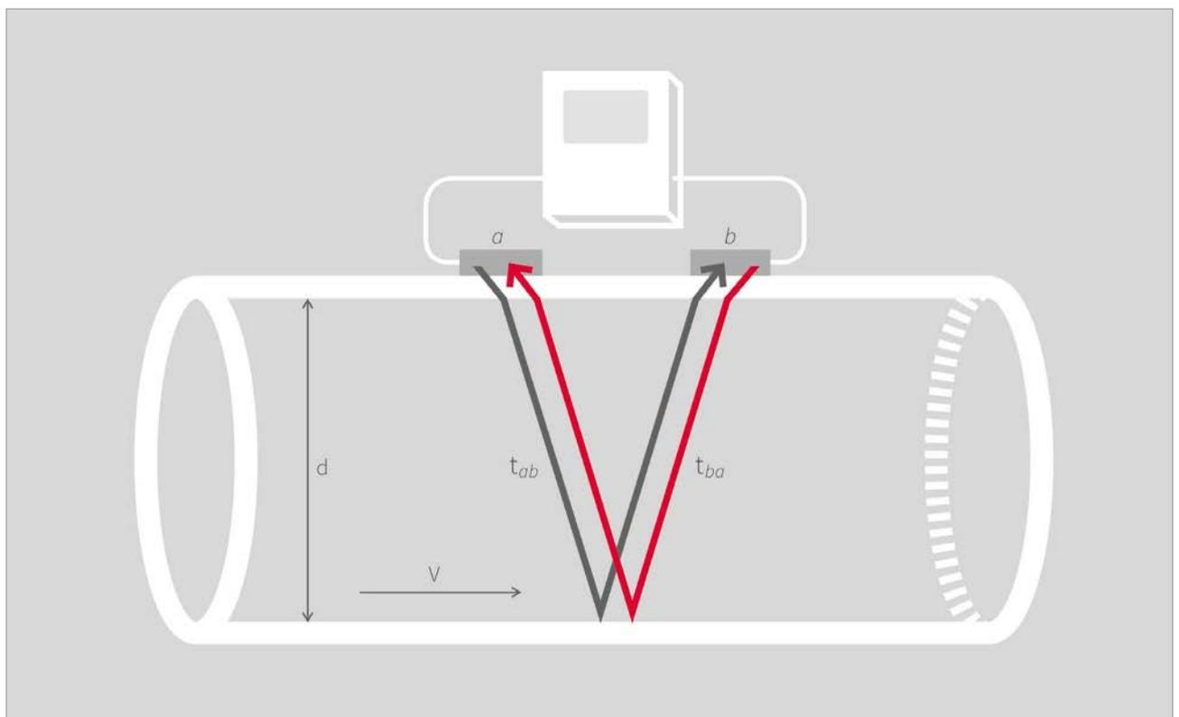
Sensors *a* and *b* work alternately to send and receive ultrasonic pulses. The sound waves *ab* travelling with the flow move faster than those travelling against it *ba*.
